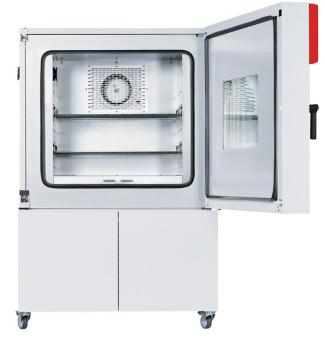
The water cooling option of the MKF humidity test chamber is now available and has the benefits of being more energy efficient due to a reduced consumption of electricity. The humidity test chamber has a greatly reduced heat output into the room the humidity test chamber is operated in thereby making it more comfortable for the operators and technicians.
